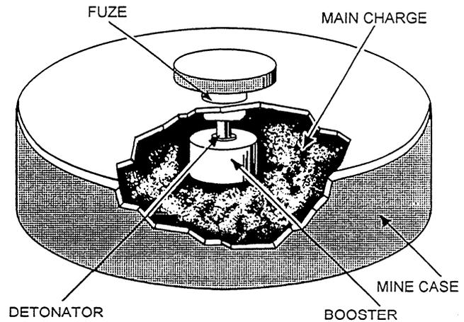
Figure 12-12.—Typical pressure type of land mine mechanism.
