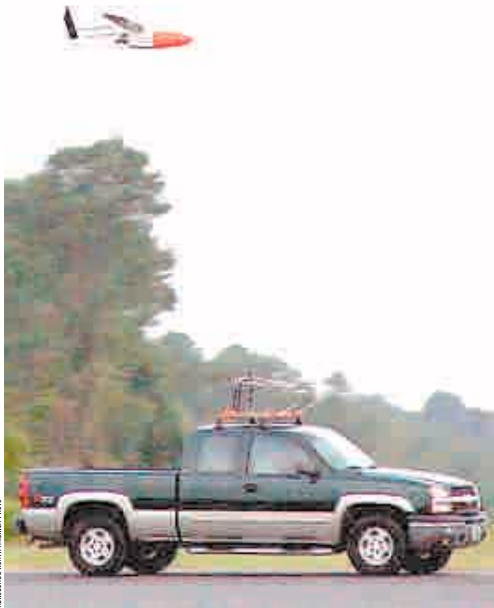
▲ An Aerosonde aircraft (like the one being launched above), equipped with meteorological sensors, GPS receivers and satellite communications gear, flew directly into the lower regions of Tropical Storm Ophelia as it churned off the Atlantic coast of the United States.
