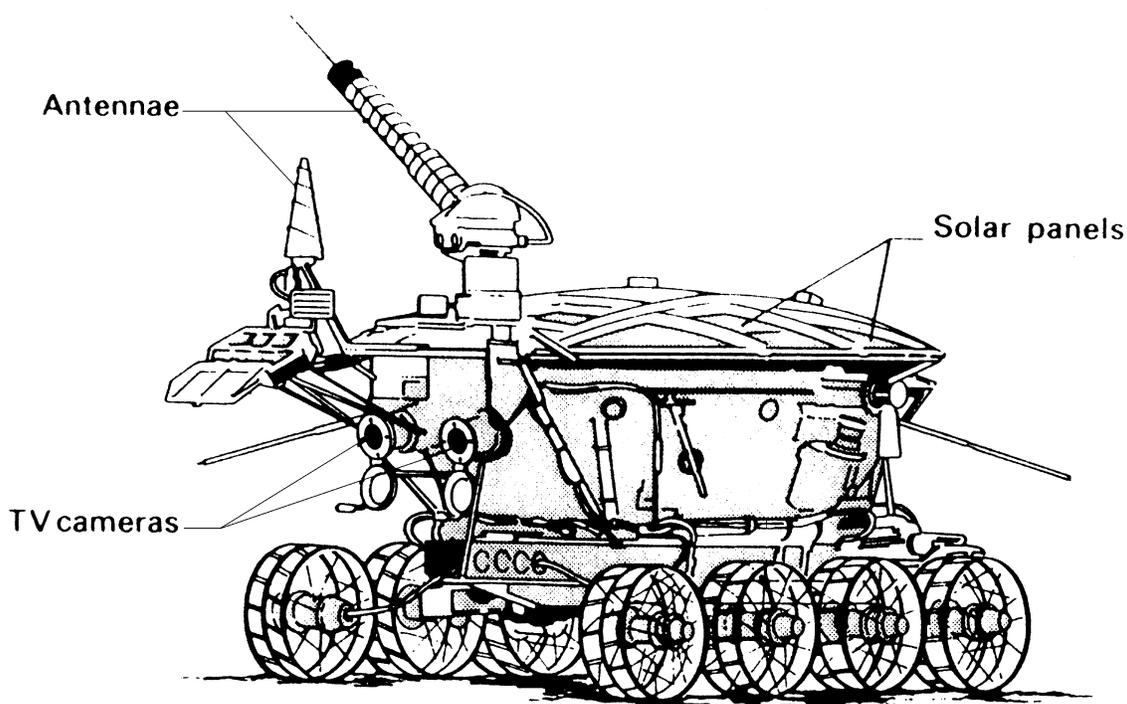
FIGURE 3.1.1 This sketch shows the basic features of the former Soviet Union Lunokhod rover. Two such vehicles were deployed on the Moon in the early 1970s. Illustration adapted from *The Moon—Our Sister Planet*, Cambridge University Press, Cambridge, England, 1981.
